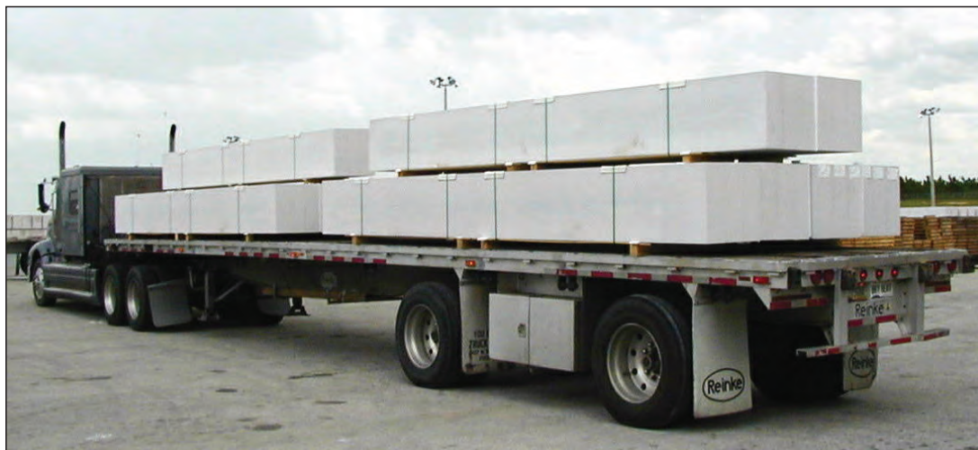
Shown here is a truck with AERCON panels. An AERCON panel weighs approximately 25% of standard cast-in-place concrete.
